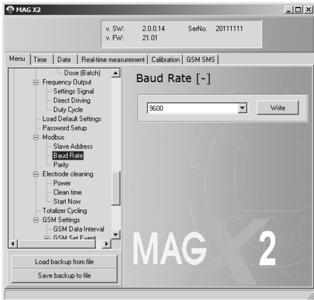
Picture 4. MODBUS communication protocol settings
