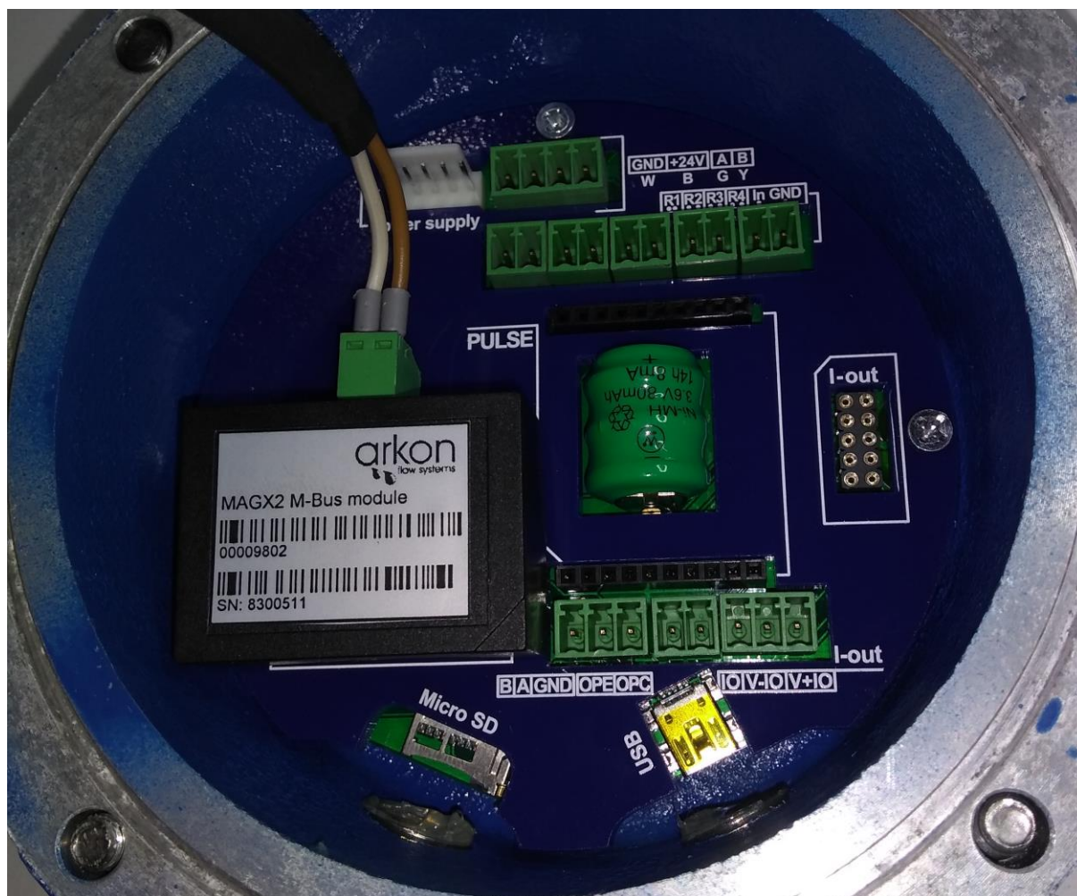
Picture 1. M-Bus module location
