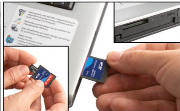
Micro SD card inserted in micro SD card adapter and plugged into the laptop card reader
