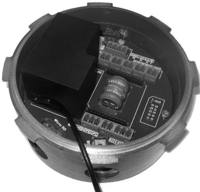
Picture 6. GPRS module location
