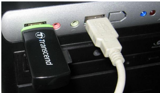
External card reader with micro SD card connected to the USB slot
