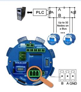
Multi-Node Network with End Termination Using RS485 Terminator R, with resistance  $100\Omega$  should be connect to the end of line RS485.
