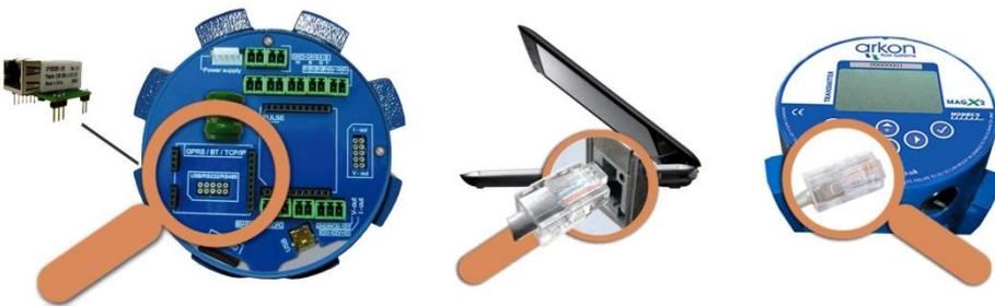
There is a condition that must be fulfilled for the TCP/IP module to be able to operate correctly: line speed of the communication protocol MODBUS must be set up on 19200Bd, Parity none, 1 stop bit. If there is a different setting the communication will not work.
