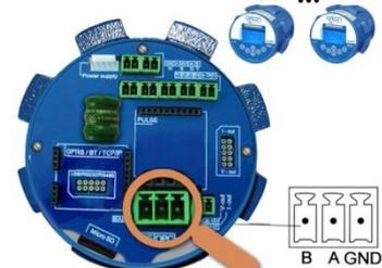
Multi-Node Network with End Termination Using RS485
