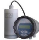
The MQU is the Arkon ultrasonic flowmeter for open channels. It should be use in combination of a flume. It is available for measurement ranges from 0.5 to 4 meters. The transmitter includes a LCD display, 4 buttons, internal data-logger, communication RS232 or RS485 (with Modbus RTU as option), temperature compensation and analogue and binary output.. There is also available a version for measurement with 2 sensors instead of 1.
