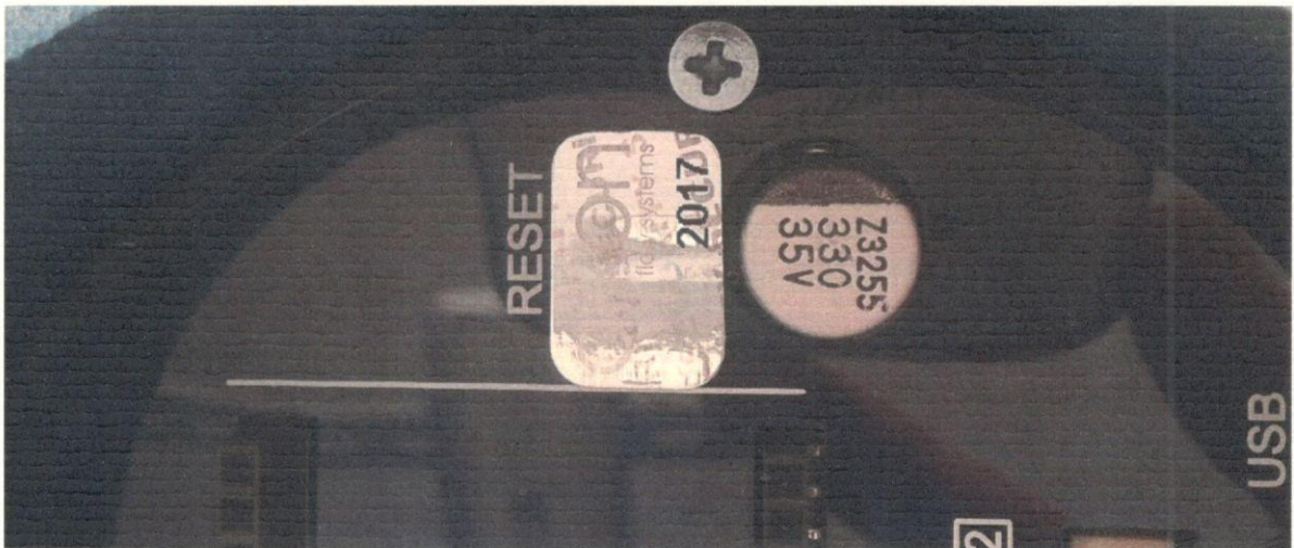
Figure 3: The water meter type MAGB1 – reset jumper:
