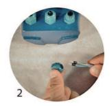
Pass the cable through screw female part of the cable gland
