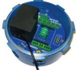
Screw the antenna and connect antenna to module
