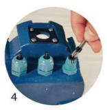
Pull the cable through the cable gland by the insulation
