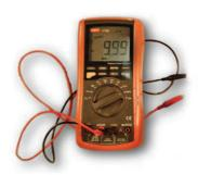
If 4-20mA Current Loop module is connected correctly, you can measure ~10mA on Output
