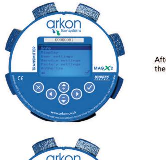
After switching on the transmitter the display should appear like this
