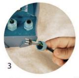
a) You must use a cable with a round cross-section
