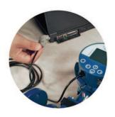
Connect cable to PC to serial RS232 communication port
