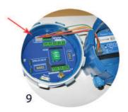
Warning: connection between the power supply module and the motherboard is protected with a lock
