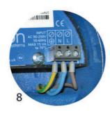
All three power supply conducts must be properly tightened
