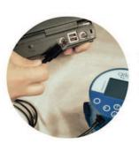
Connect transmitter to PC with standard USB cable
