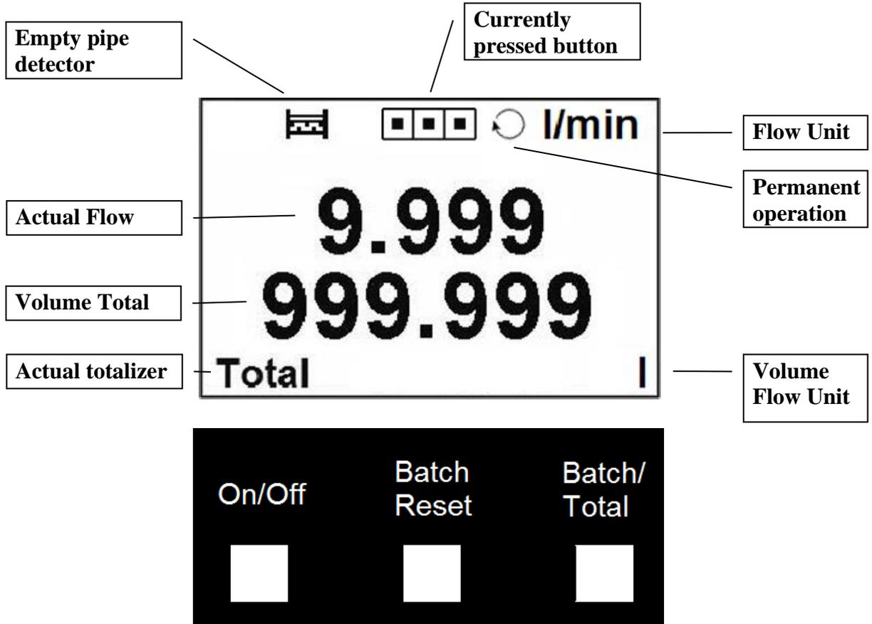
**Note:** these are not pushing buttons, to activate hold your finger over the white rectangle for 2 to 4 seconds.
