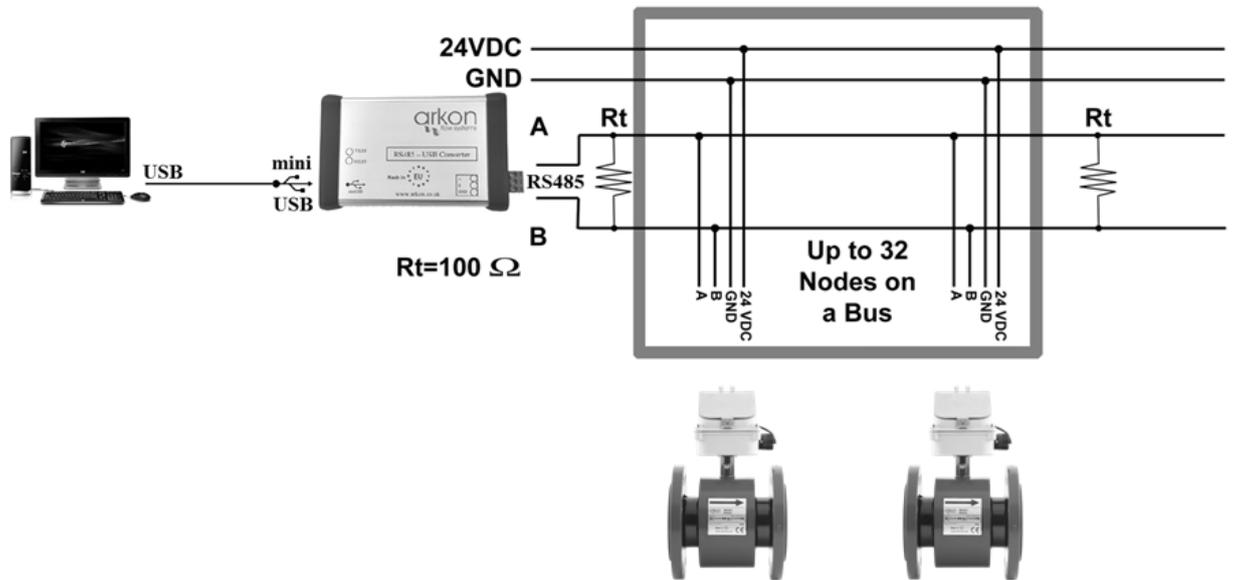
Picture above shows practical connection MAGE1 to PC through USB using RS485 – USB Converter.
