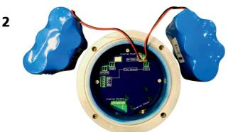
2. Unplug the old battery pack, remove it from the transmitter and replace with the new battery pack.
