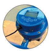
Connect the miniUSB cable to the transmitter
