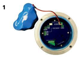
1. Connect the new battery pack to the second battery connector (Picture 2 - without losing measurement data).
