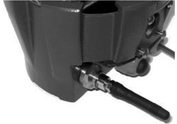
Picture 2. Antenna and GPRS battery installation
