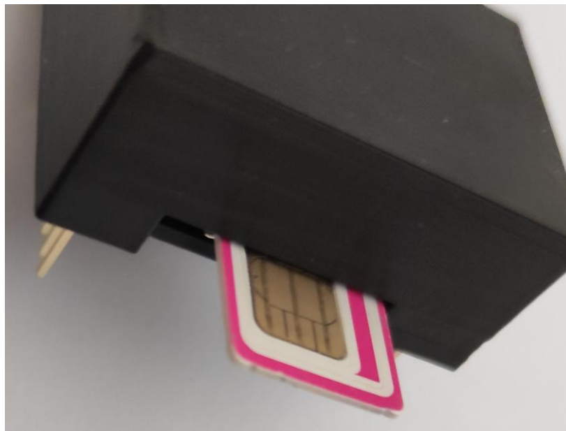
Picture 1. SIM card installation into the 3G/GPRS/GSM Module
