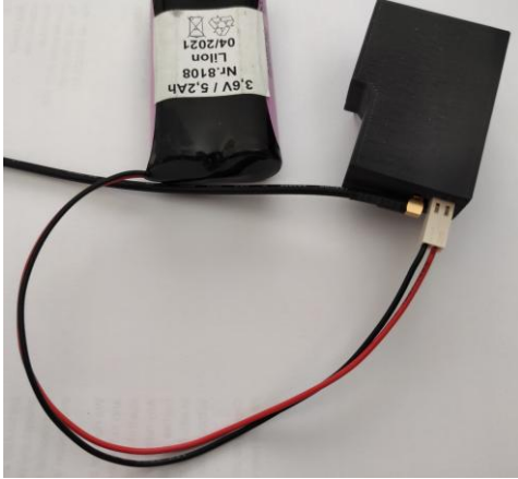
Picture 2. Antenna and GPRS battery installation
