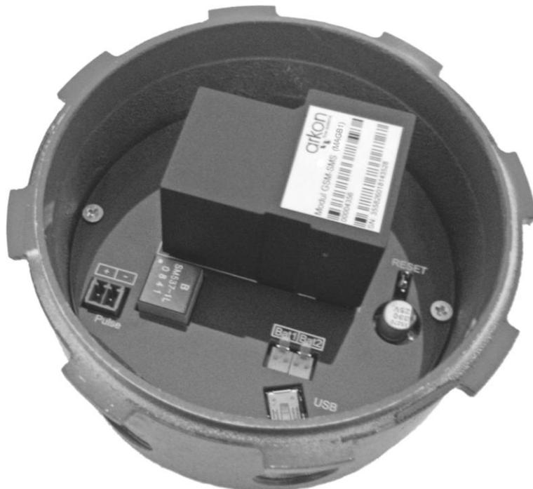
Picture 3. Install 3G/GPRS/GSM Module into the transmitter
