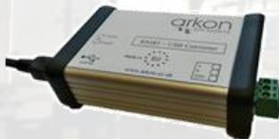
Allows to connect any RS485 communication based device directly to USB.
