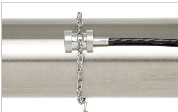
PT100 transducer fixed to pipe
