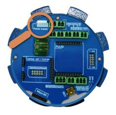
Recommended power supply cable minimum  $3xØ1mm^2$ All used wires have to be round crosscut cables.
