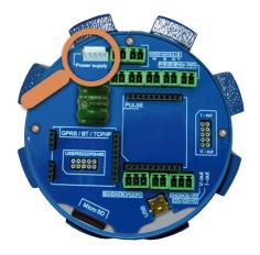
Recommended power suplly cable minimum  $2x\emptyset0.5 mm^2$  All used wires have to be round crosscut cables.
