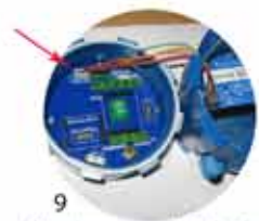
9 Warning: connection between the power supply module and the motherboard is protected with a lock.
