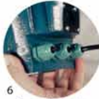
6 Screw the female part to cable gland.
