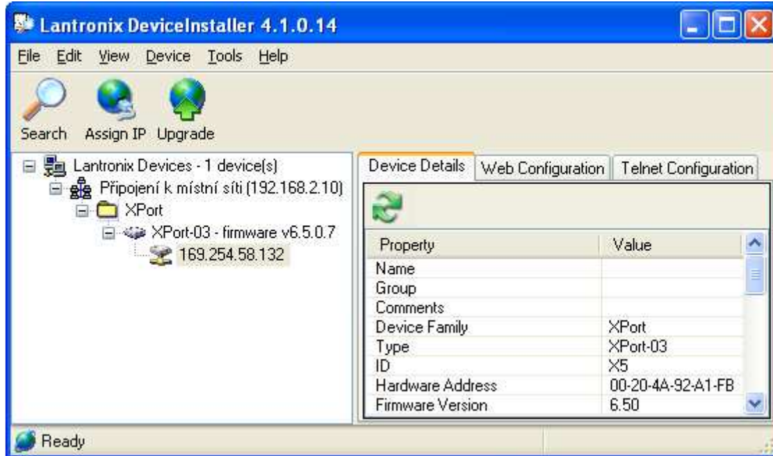
Fig. 5: You can change the IP address click on the Assign IP icon
