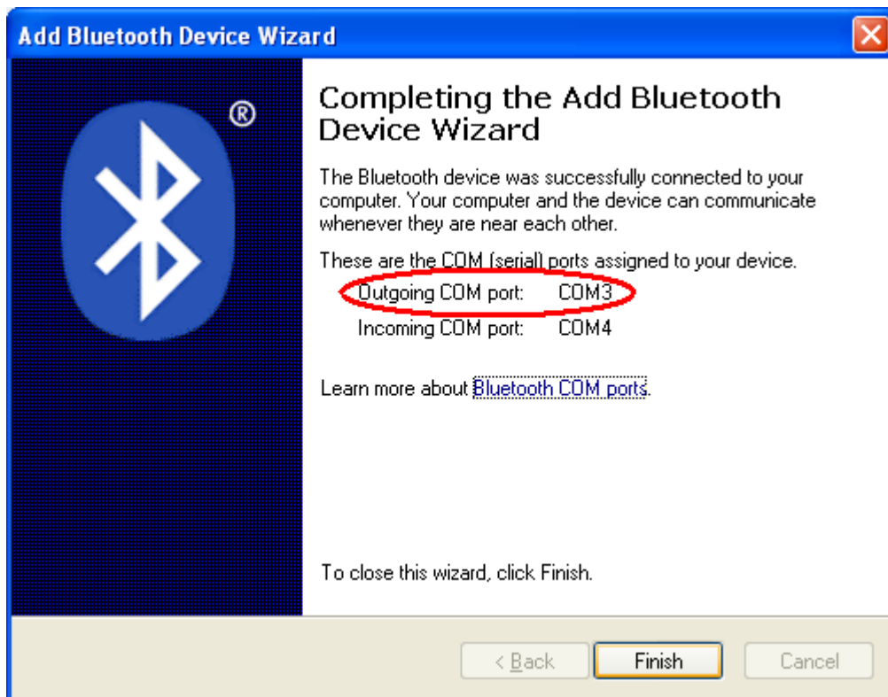
Fig. 7: Computer and this Flowmeter can communicate via Outgoing COM3 port.
