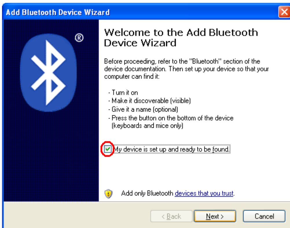
Fig. 4: Check 'My devices is set up and ready to be found' and click on Next
